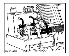
NOTE: Clean spills at once. Cap all hoses immediately to prevent contamination of the hydraulic system.
